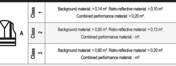
The coefficient of retro-reflection of the retro-reflective material must be class 2 to comply with EN ISO 20471 (class 1 of previous EN 471 standard has been cancelled). «X» indicates the class of the garment according to the compulsory minimum area..
