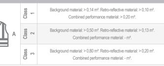
The coefficient of retro-reflection of the retro-reflective material must be class 2 to comply with EN ISO 20471 (class 1 of previous EN 471 standard has been cancelled). «X» indicates the class of the garment according to the compulsory minimum area..
